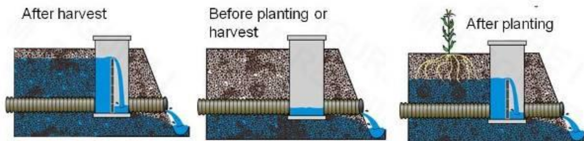
Figure 6.4 Drainage management practices allow farmers to drain only as needed (Source: Purdue University)
